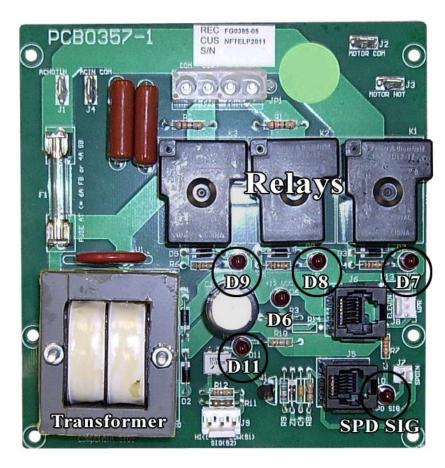
**D6** - Main power indicator. This light should be lit when the treadmill is plugged in, even if the treadmill is not turned on.
